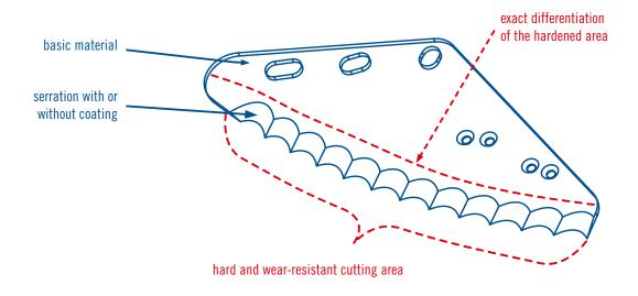
Due to the use of special alloy tool steel, which is very hard and wear-resistant, **Busatis quality knives for balers and self-loading wagons** achieve a very high level of cutting performance and long intervals between grinding.
